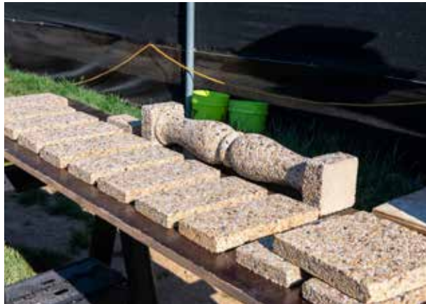
Left: Reproducing mosaic concrete required evaluating materials, molds, placement, and finishes. These precast mosaic concrete samples were evaluated onsite to assure consistency of appearance. Photo by Hank Davis.
